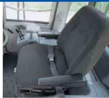
Deluxe suspension seat The cloth-covered seat offers both comfort and suspension.
