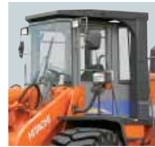
Outer ROPS/FOPS* cab This rigid cab is ready "just in case" to help protect the operator from falling objects or during a rollover. The rear-hinged door makes entry and exit easy.
