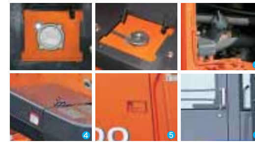
1 Fuel cap 2 Hydraulic fluid cap 3 Transmission fluid cap 4 Battery box 5 Side cover 6 Cab door
